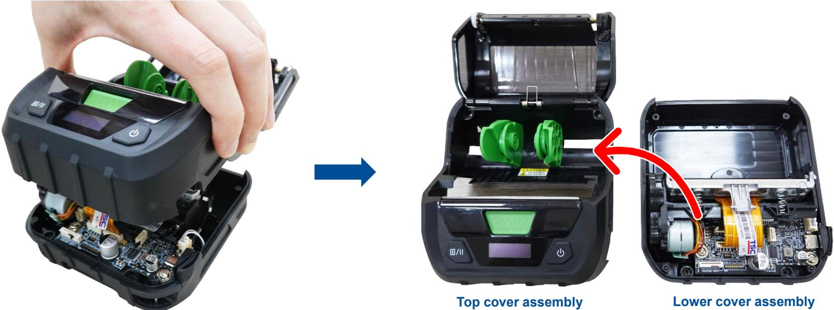
6. Carefully detach the flat cable from the top cover assembly.
