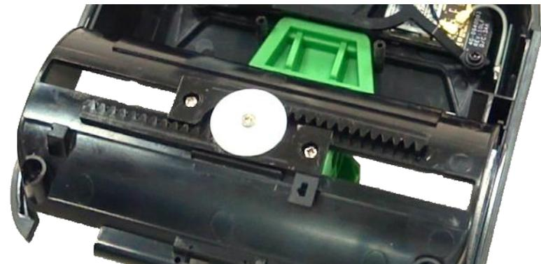
4. Use the #1 Phillips screwdriver to remove two screws on the gear bars for media holder.
