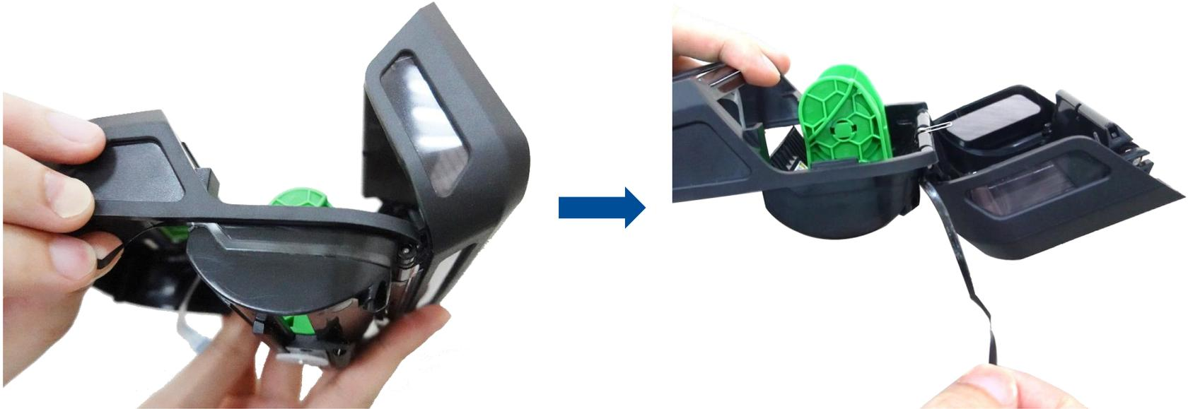
7. Pull the shaft out after pushing it out of the chassis with a tool.
