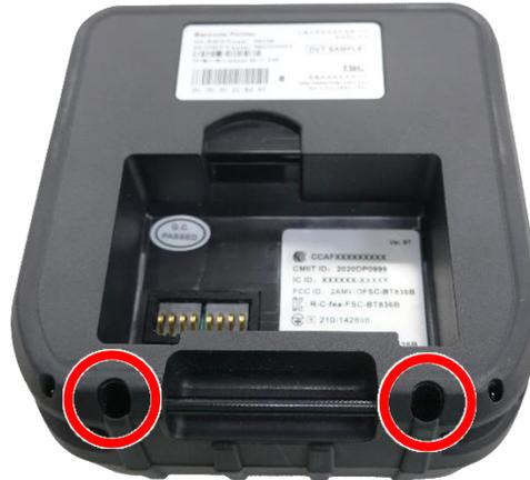
3. Open the media cover. Remove two screws on lower inner cover.
